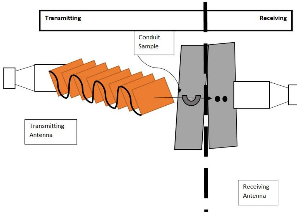
The test setup is the same as other shielding effectiveness, first determining the dynamic range of the unit/sample and the actual measurement of the signal for the sample in question.
