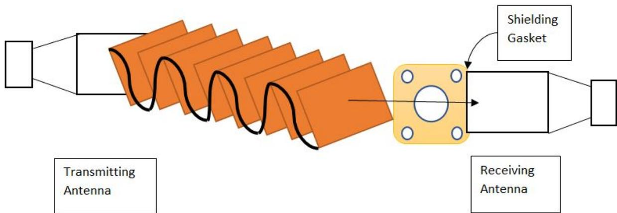
Measurements are made using the plane wave shielding effectiveness method. The gasket will be determined by its ability to electrically bond a test cover panel to an enclosure flange so the radiated RF plane wave will attenuate through a 24-by-24-inch opening. The enclosure needs to be large enough so no part of the transmitting antenna is within one meter of any enclosure surface.
