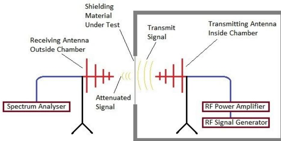
As a verification of results, there is a step prior step to the actual measurement of the sample under test. This step requires a calculation of the dynamic range such that accurate results are being made. Therefore, two measurements must be made.
